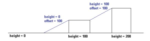
The height of a ramp is where it starts (the lowest point), the offset of a ramp is always a relative value! (the highest point – but not as an absolute value).
